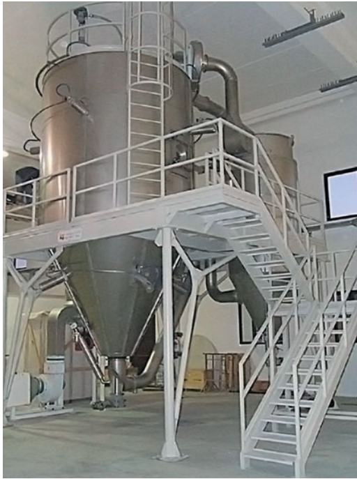
Figure 36.1 Spray dryer. Industrial spray dryers are used to dry or concentrate large volumes of high-value liquid foods.
