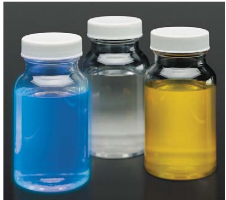
Figure 35.3 The IDEXX Colilert water quality test system. Colilert reagents are added to 100-ml water samples. After incubation for 24 h at 35–37°C, the samples develop yellow color if they contain coliform bacteria (right). Samples containing Escherichia coli develop yellow color and also develop blue fluorescence (left). Samples negative for coliform bacteria remain clear (center).
