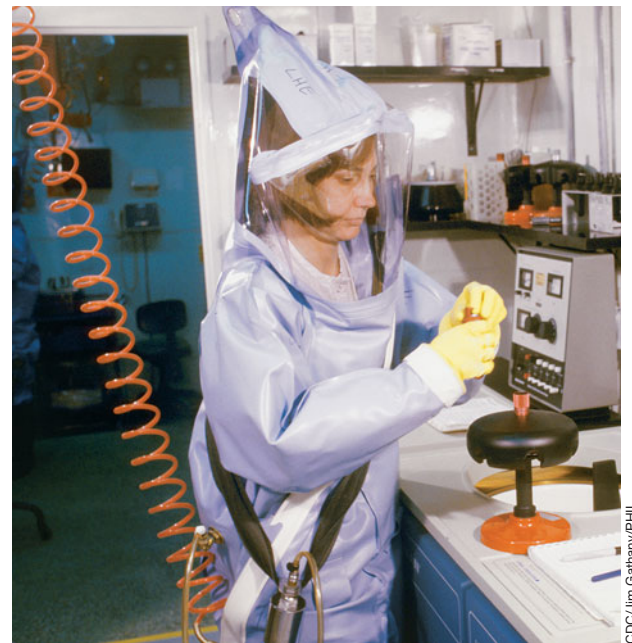
Figure 31.9 A worker in a BSL-4 (biological safety level 4) laboratory. BSL-4 is the highest level of biological control, affording maximum worker protection and pathogen containment. The worker has a whole-body sealed suit with an outside air supply and ventilation system. Air locks control all access to the laboratory. All material leaving the laboratory is autoclaved or chemically decontaminated.
