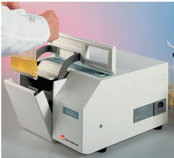
Figure 36.10 A stomacher. Paddles in this specialized blender homogenize the solid food sample in a sealed, sterile bag. The sample is suspended in a sterile solution.
