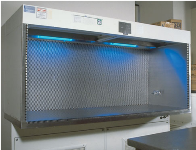
Figure 26.4 A laminar flow hood. An ultraviolet light source prevents contamination of the hood when it is not in use. When in use, air is drawn into the cabinet through a HEPA filter. The filtered air inside the cabinet is exhausted out of the cabinet, preventing contamination of the inside of the hood. The cabinet provides a contaminant-free workspace for microbial and tissue culture manipulations.
