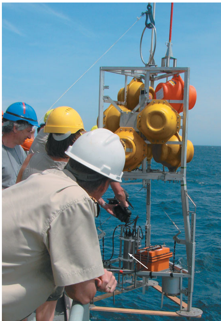
Figure 22.21 Deployment of deep-sea lander. The lander is equipped with a bank of microelectrodes (arrow) to measure distribution of chemicals in marine sediments.
