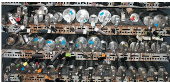
Figure 23.28 Pressure cells for growing piezophiles under elevated pressure. (a) Photo of several pressure cells incubating in a cold room (4°C). (b) Schematic design of a pressure cell. These vessels are designed to maintain pressures of 1000 atm.
